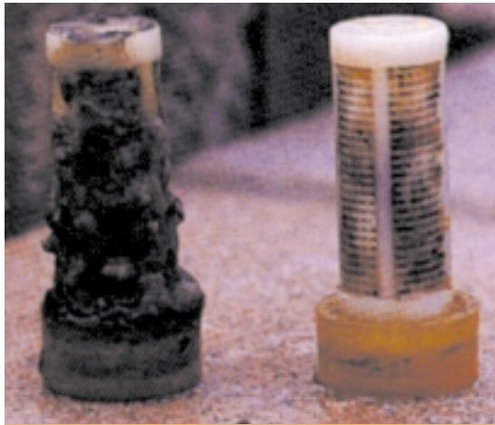
Figure 5. Dirty Filter (left); cleaned filter (right)
